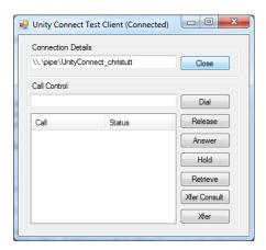
Otherwise an error message will be displayed if the connection attempt failed. The most likely reason for the connection attempt to fail is that the pipe isn't given the connect name or the named server isn't enabled in Unity. In either case go to Settings in Unity and check that UnityConnect is enabled, then ensure that the named pipe in the sample client is the same as the named pipe that Unity Connect is listening on.
