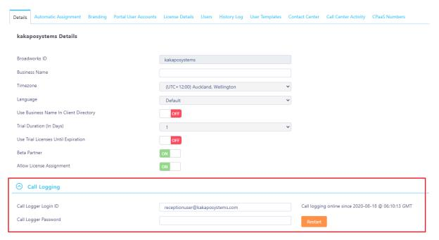
If there was an issue and the engine couldn't automatically reconnect, then you can manually restart the logger instance by clicking the Restart button shown above.
